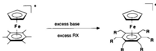
Scheme 2. Hexaalkylation of [\text{FeCp}(\text{C}_6\text{Me}_6)]^+ (R = alkyl, e.g., CH 3 ; CH 2 Ph).
